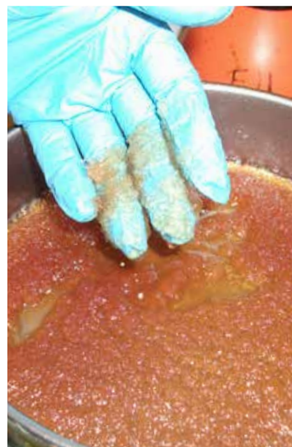
Fig. 13: Waxy precipitations in a fuel sample
